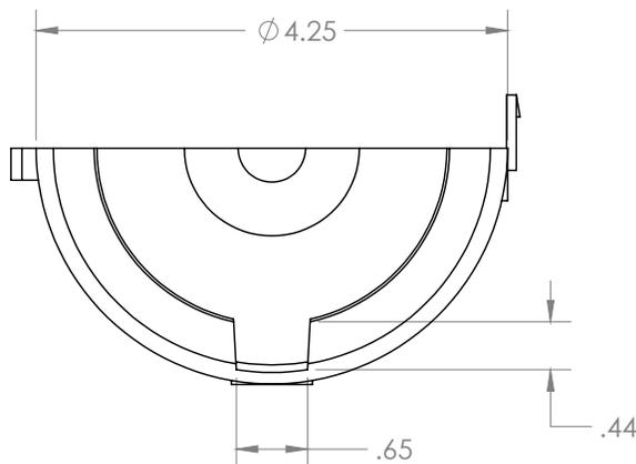
Durability in wildlife protectors is defined by its material, wall thickness, latching system and U.V. resilience. RMC Plastics combines our Positive Latching System, heavy-duty wall thickness (over 100 thousands of an inch), and superior U.V. protection to meet these challenges.
