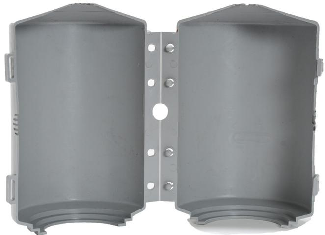
RMC Plastics introduced the SG-580 in 1995 as a more economical option for our customers. A one-piece folding guard, this unit is simple to install and has a large enough diameter to fit almost all bushing sizes being used today. The bottom-ring diameter can be made larger simply by trimming away one of the sizing rings.
