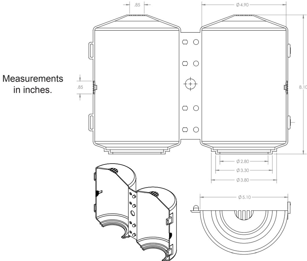
Durability in wildlife protectors is defined by its material, wall thickness, latching system and U.V. resilience. RMC Plastics combines our Positive Latching System, heavy-duty wall thickness (over 100 thousands of an inch), and superior U.V. protection.
